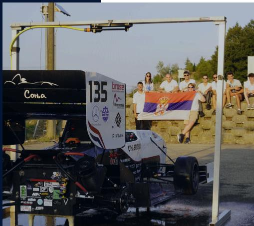
**The rain test** simulates driving in the rain – the vehicle is sprayed with water to check the insulation of the electrical systems.
